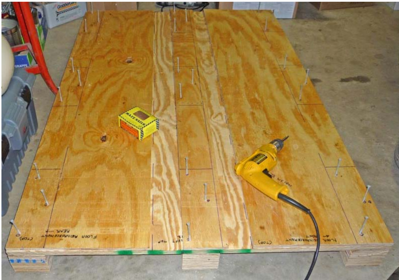
Caption: The floor of the crate is 1.25" thick.
