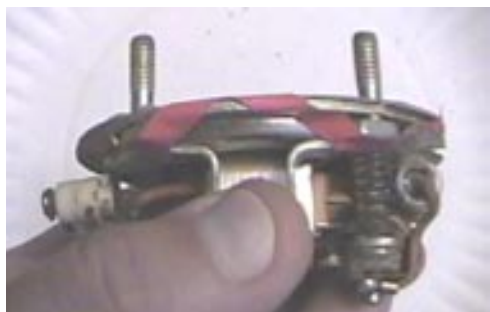
Figure 5 Tape holding mounting posts
