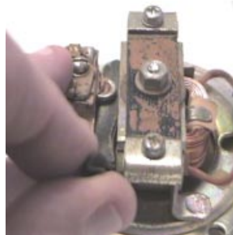
Figure 4 Sandpaper between points
