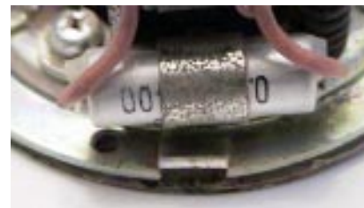
Figure 3 Location of locking tab
